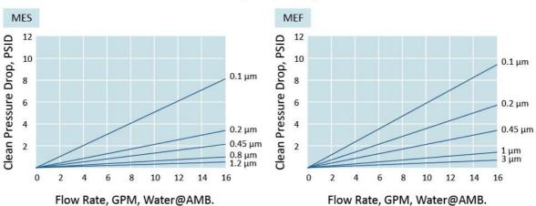
Flow rate is per 10" cartridge. For liquids other than water, multiply the pressure drop by the fluid viscosity in centipoises
